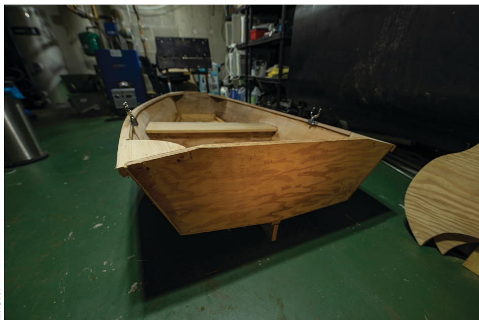
The stern of the unfinished but well underway little pram. A set of oarlocks ("rowlocks" in the UK) convey some dignity.
